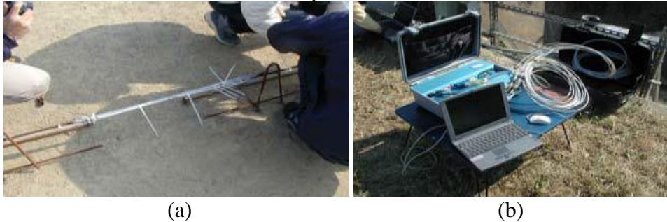
Figure 7. (a) SOFO Optical Fiber Sensor, (b) DAS System [21],
