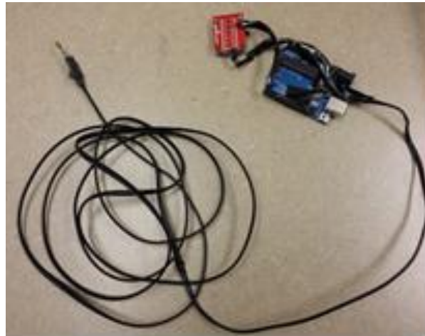
Figure 7: Wireless transmission end without batteries
