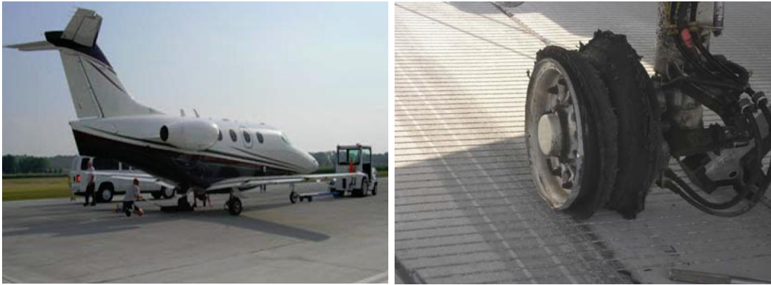
Figure 2. Damaged Aircraft in Ankeny Regional Airport Runway [7]
