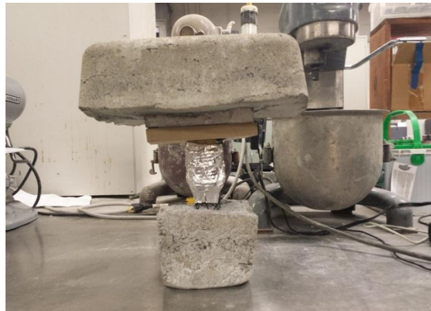
Figure 12: Wireless MEMS system inside concrete
