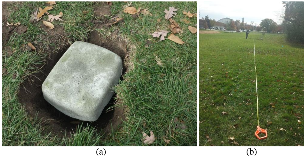
Figure 4-9. Success rate test: (a) wireless MEMS system inside concrete buried underground; (b) vertical distance measurement for data transmission.
