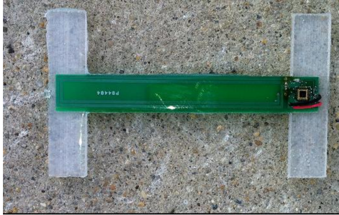
Figure 8. Prototype Installation of Self-powered Strain Sensor [22]
